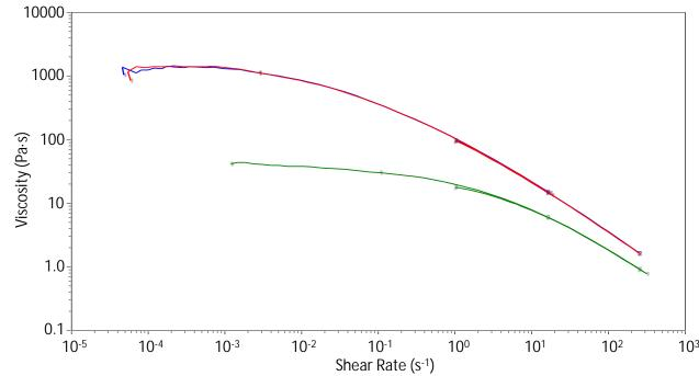
RHEOLOGY: Viscosity of the DuoGel formulations: FID 3000 (Blue), FID 3001 (Green), and FID 3002 (Red). The gel formulations were evaluated under both a sheer stress sweep and a shear rate sweep.
