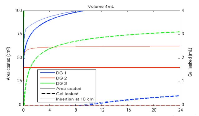
Spreading of three different DuoGel formulations: DG1 (blue – gel viscosity of 71 Pa·s at 1 s<sup>-1</sup> shear rate), DG2 (red – gel viscosity of 178 Pa·s at 1 s<sup>-1</sup> shear rate), and DG3 (green – gel viscosity of 8 Pa·s at 1 s<sup>-1</sup> shear rate). Four milliliters of the gel was inserted mid-vagina (10 cm) and the area covered by the gel (solid line) vs. volume of gel that leaked (dashed line) was evaluated for 24 hours.
